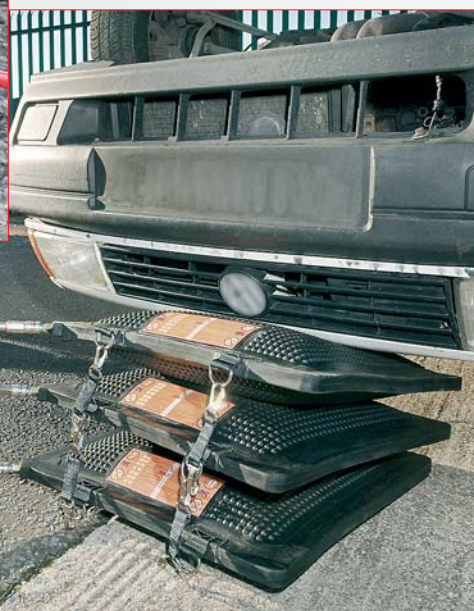
Several high-pressure air cushions may be connected to each other.
