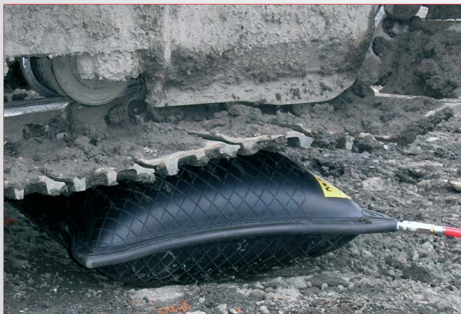
Several high-pressure air cushions may be connected to each other.
