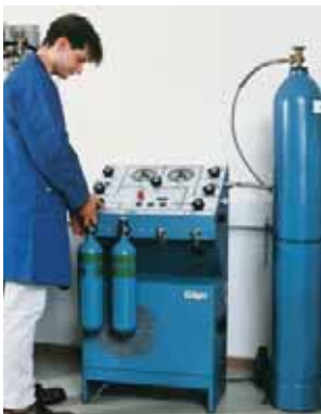
Dräger Oxygen Booster DOB 200: Filling process
